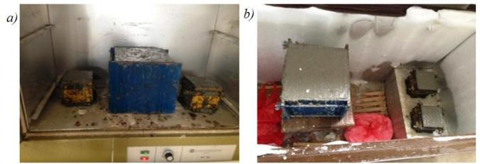
Figure 1. Samples exposed to high temperatures in the furnace (+60°C) (a) and low temperatures in the freezer (-20°C) (b)
