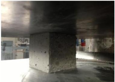
Figure 2. Strength tests on the concrete sample, after a period of care
